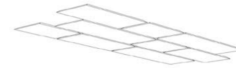
ceiling fixed with glue
